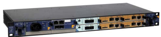
Compact TORNADO-MTCA® DSP/FPGA modular system with four TORNADO-A6678 DSP/FPGA M/S AMC-modules and two T/AX-DSPX network AMC-modules in 19" 1U 6-slot MicroTCA® chassis with 10GbE backplane switch
