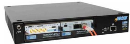
Mini TORNADO-mMTCA® DSP modular system including TORNADO-AZ/FMC AMC-module with FMC A/D submodule and T/AX-DSPX AMC-module with 10GbE SFP+ ports all installed into dual-slot MicroTCA® mini chassis with passive backplane
